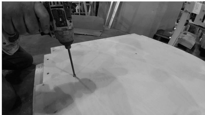
▲ Ensure the 6 Flat Head Machine Screws are firmly fastened.
