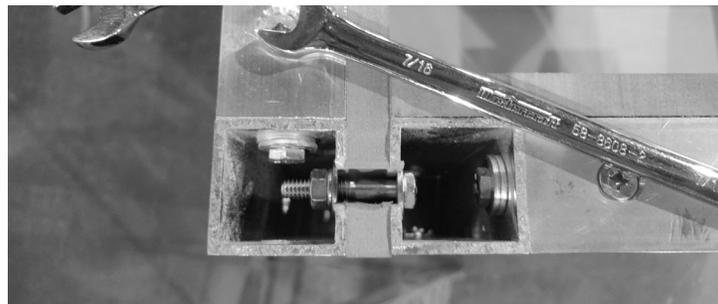
▲ ENSURE TO KEEP SAME BOLT CONFIGURATION AS SHOWN IN THE IMAGE ABOVE.
