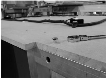
▲ ENSURE THAT THE HEX BOLTS ARE SECURELY FASTENED TO THE THREADED INSERTS.
