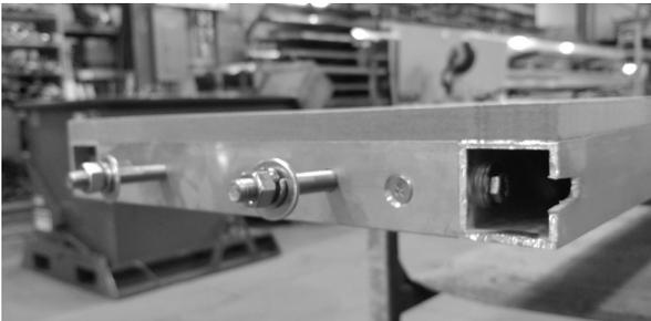
▲ UNDERSIDE OF THE B1 PANEL. ENSURE TO REMOVE THE NUTS AND WASHERS PRIOR TO INSTALLING THE B1 PANEL.
