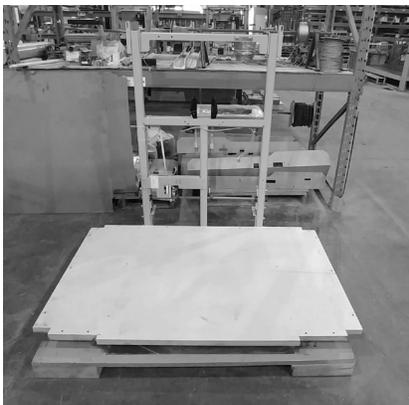
▲ Ensure the floor is properly positioned and the screw holes are aligned.
